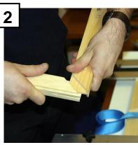
3. When you have assembled the four sides together insert the **TWO** wooden wedges that are provided to secure and strengthen each corner of the frame.
